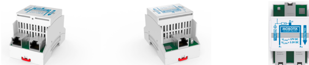
Connections on the Mx-A-SPA-HR (two views of device): 2 RJ45 to the switch (for two PoE devices) and 1 RJ45 (to the patch panel)
